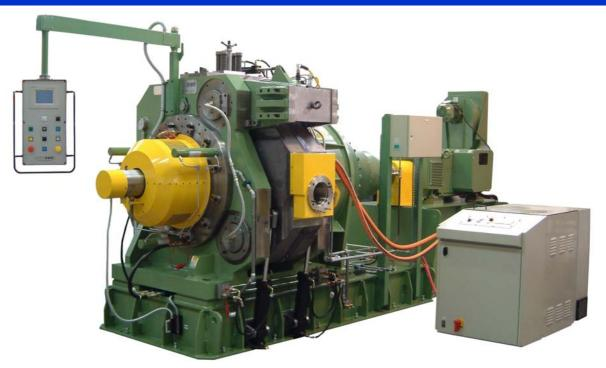
The **Conform 550i** machine is the largest of the BWE range and is capable of extruding large products such as **Copper Bus Bars / Copper Sections and Large Aluminium Sections / Profiles.**
