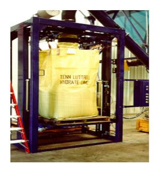
Materials of specific sizes can be automatically dispensed into a variety of storing or shipping containers.
