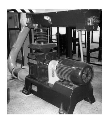
The 0,6cm granules are stored in a bin and fed to each powderizer via an independent feed screw. Once the material is reduced sufficiently, it is removed from the powderizer via vacuum pneumatics and conveyed on to fiber separation equipped with aspirators, efficiently removing the remaining fiber.
